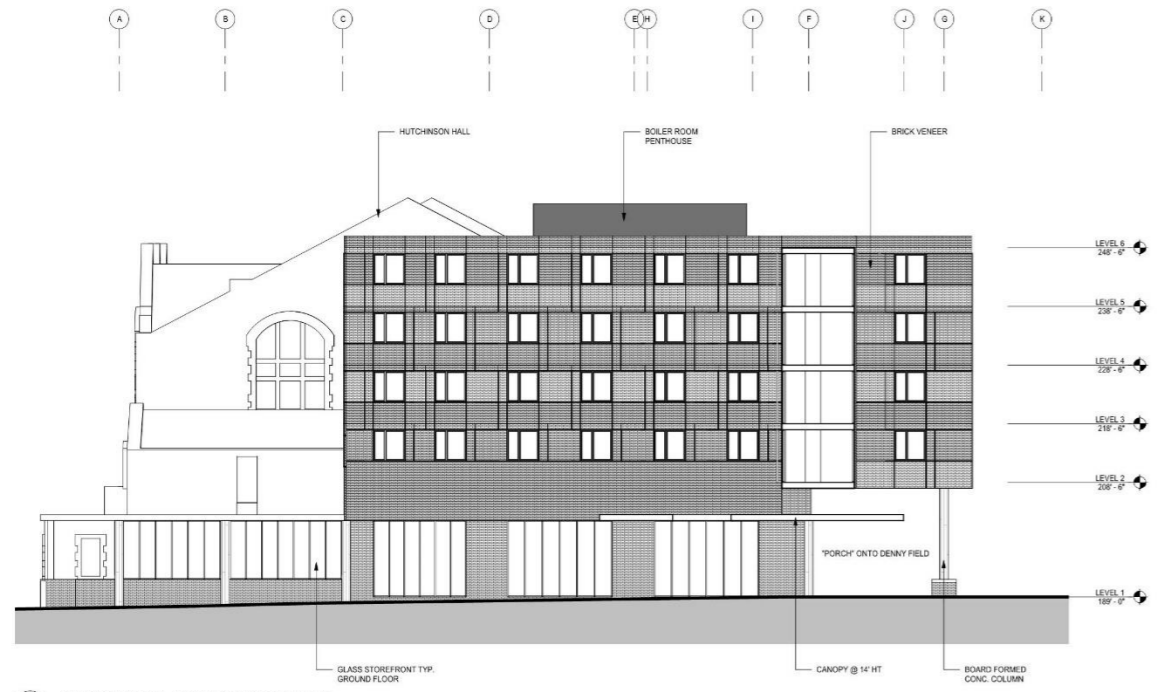
2 BUILDING ELEVATION - WEST WING FROM CHELAN LANE 3/32" = 1'-0"
