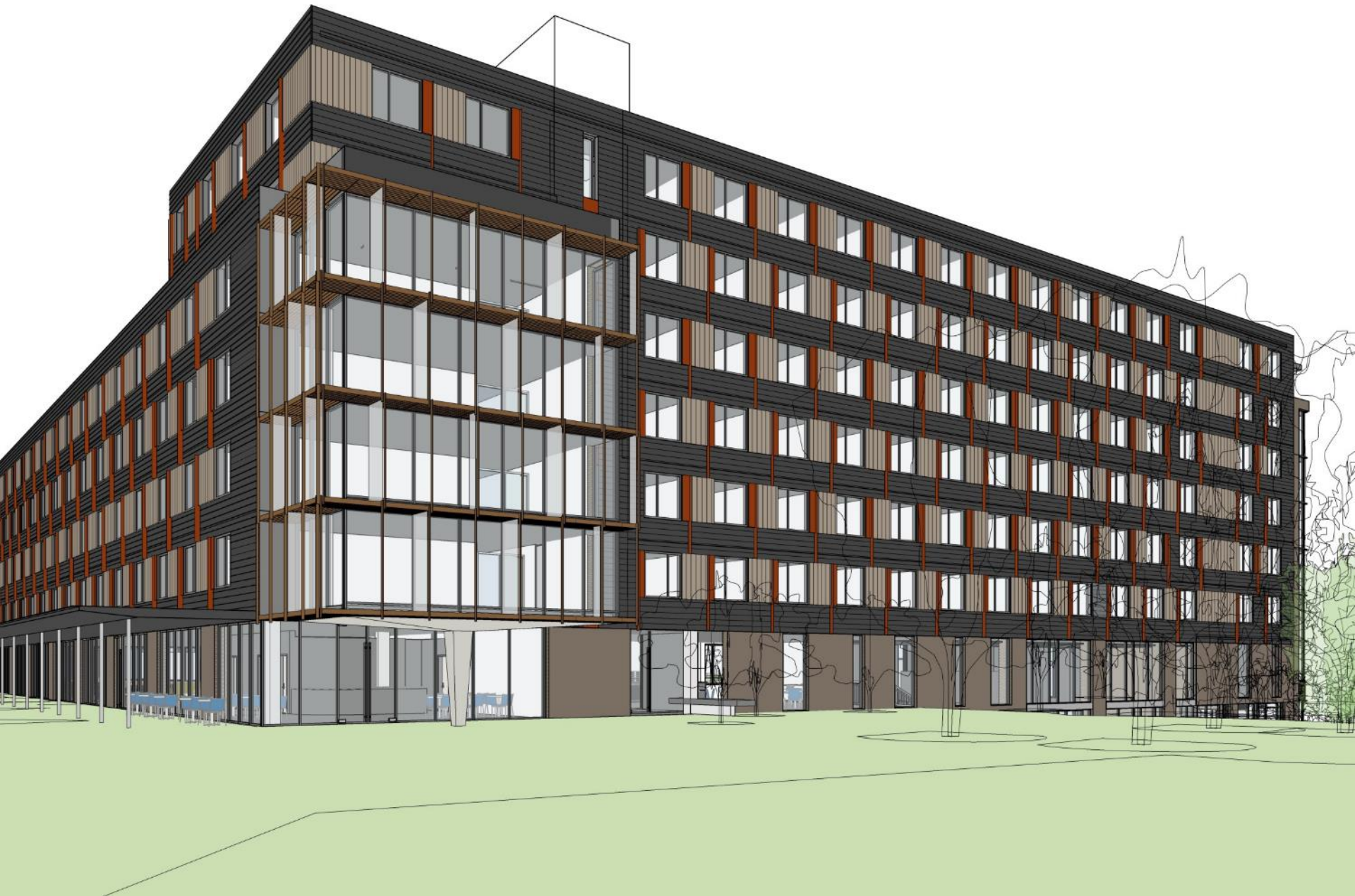
FAÇADE OPTIONS FIELD CONDITION PERSPECTIVE FROM TOWN SQUARE – METAL, WOOD INFILL SCHEME UNIVERSITY OF WASHINGTON NORTH CAMPUS HOUSING
