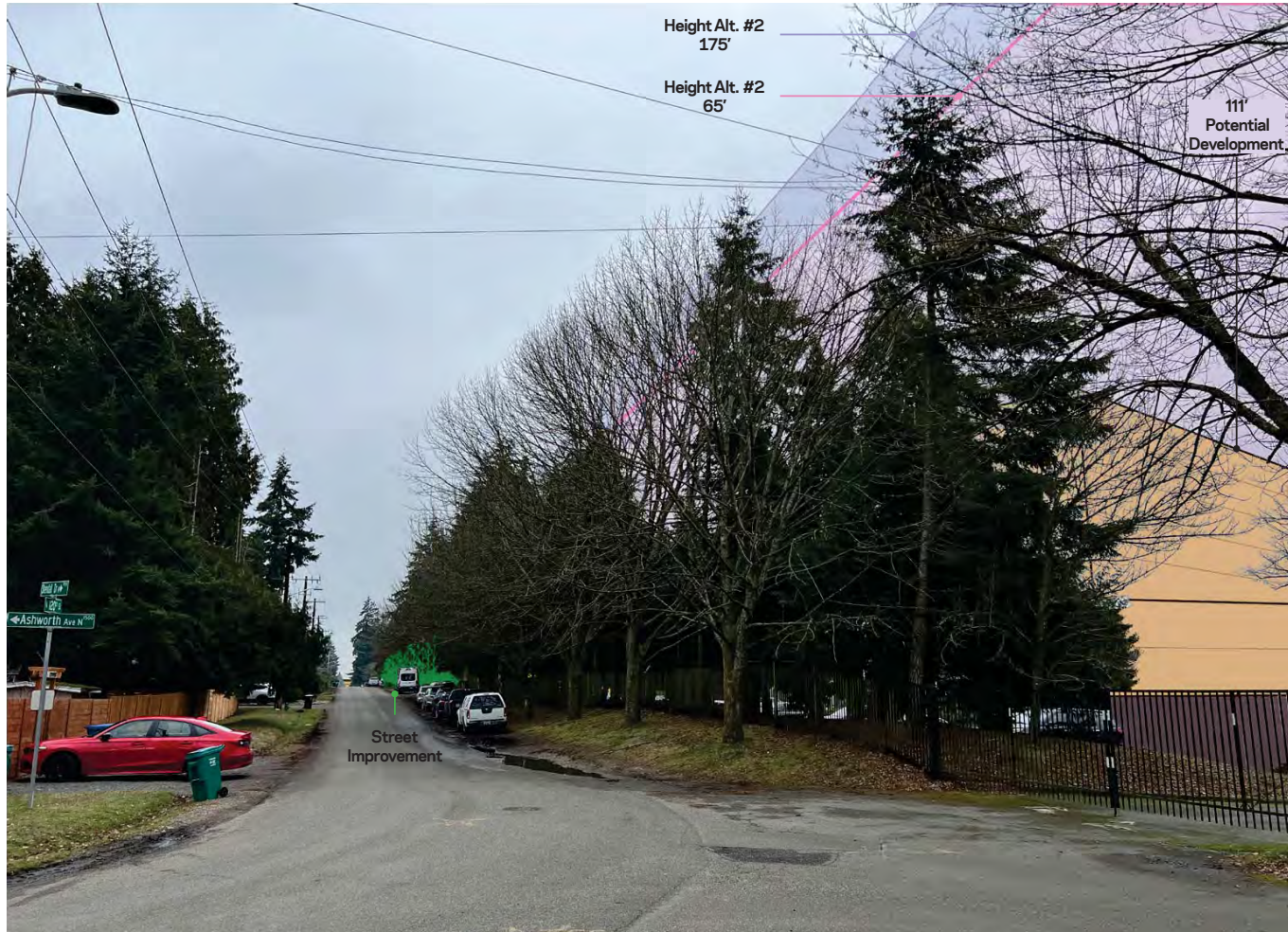
65' HEIGHT OVERLAY @ 40' SETBACK EAST FROM PROPERTY LINE; @ 60' SOUTH FROM CAMERA 175' HEIGHT OVERLAY @ 130' EAST FROM CAMERA (APPROX. 120' EAST FROM PROPERTY LINE) POTENTIAL DEVELOPMENT ALMOST 260' SOUTH FROM CAMERA
