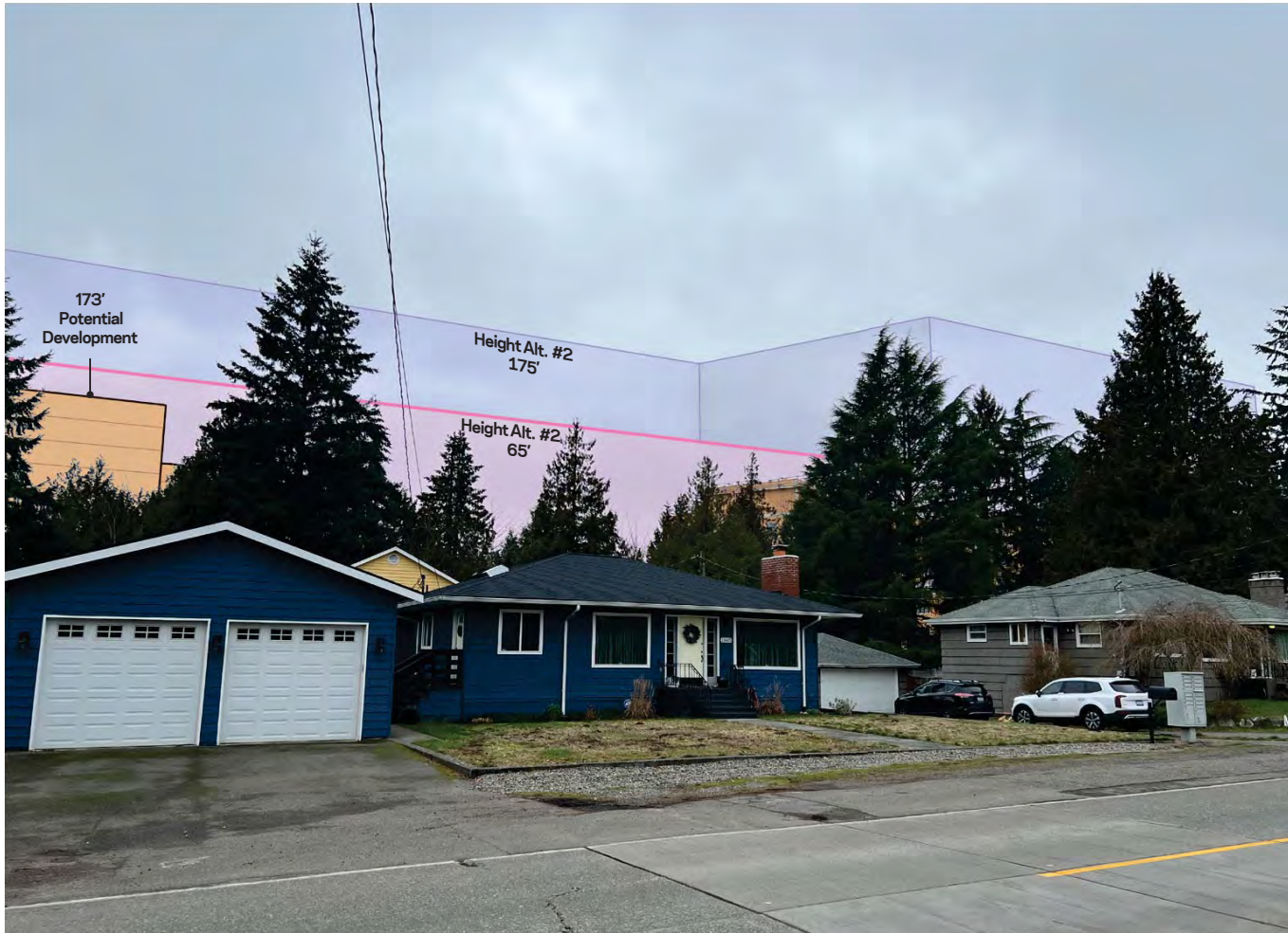
65' HEIGHT OVERLAY @ 30' SETBACK FROM PROPERTY LINE, @ 240' FROM CAMERA 175' HEIGHT OVERLAY @ 490' FROM CAMERA (APPROX. 280' FROM PROPERTY LINE) POTENTIAL DEVELOPMENT ALMOST 730' FROM CAMERA
