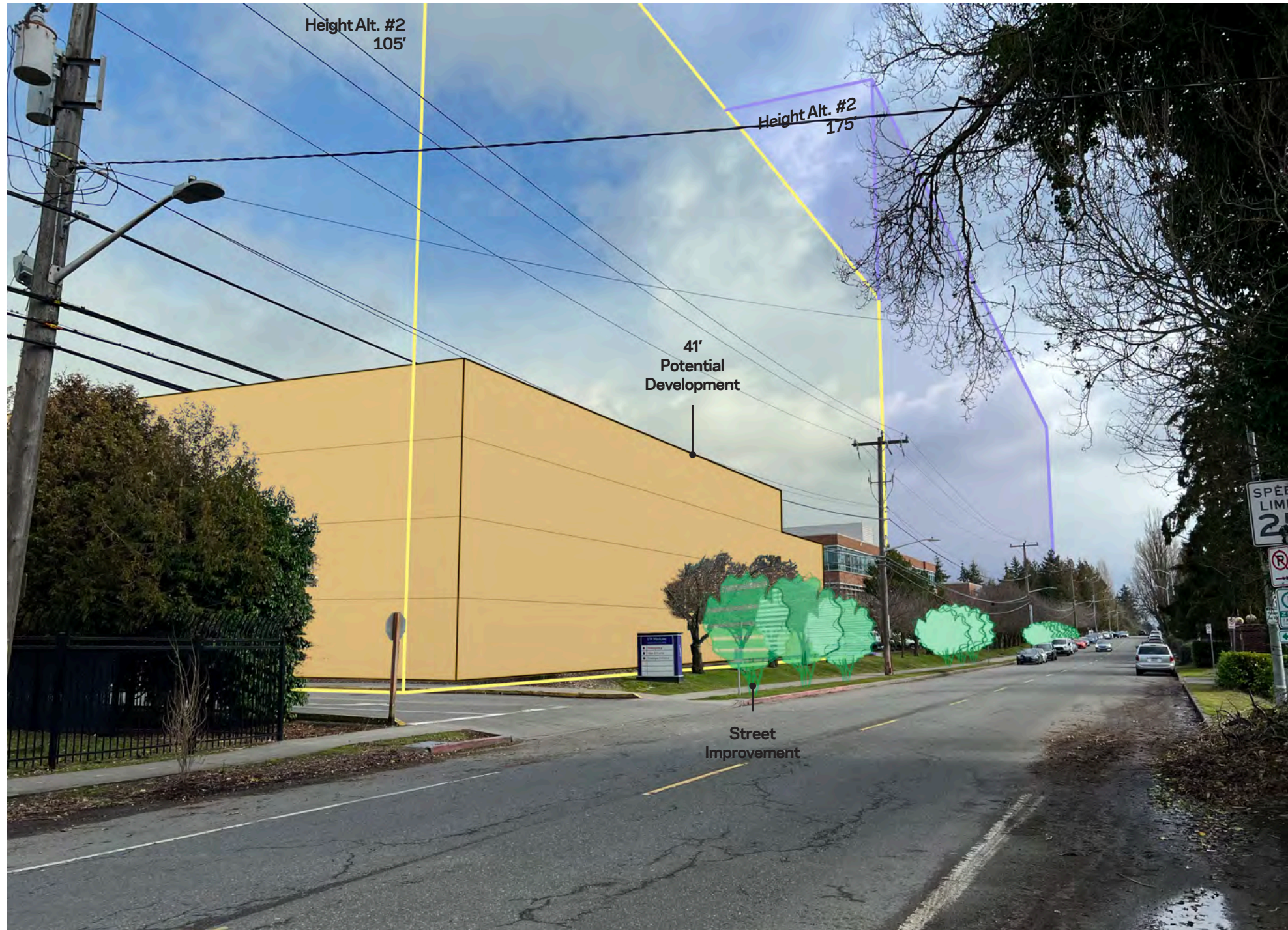
100' HEIGHT OVERLAY @ 90' EAST FROM CAMERA (APPROX. 30' EAST FROM PROPERTY LINE) 175' HEIGHT OVERLAY @ 310' EAST FROM CAMERA (APPROX. 250' EAST FROM PROPERTY LINE) POTENTIAL DEVELOPMENT ALMOST 110' EAST FROM CAMERA
