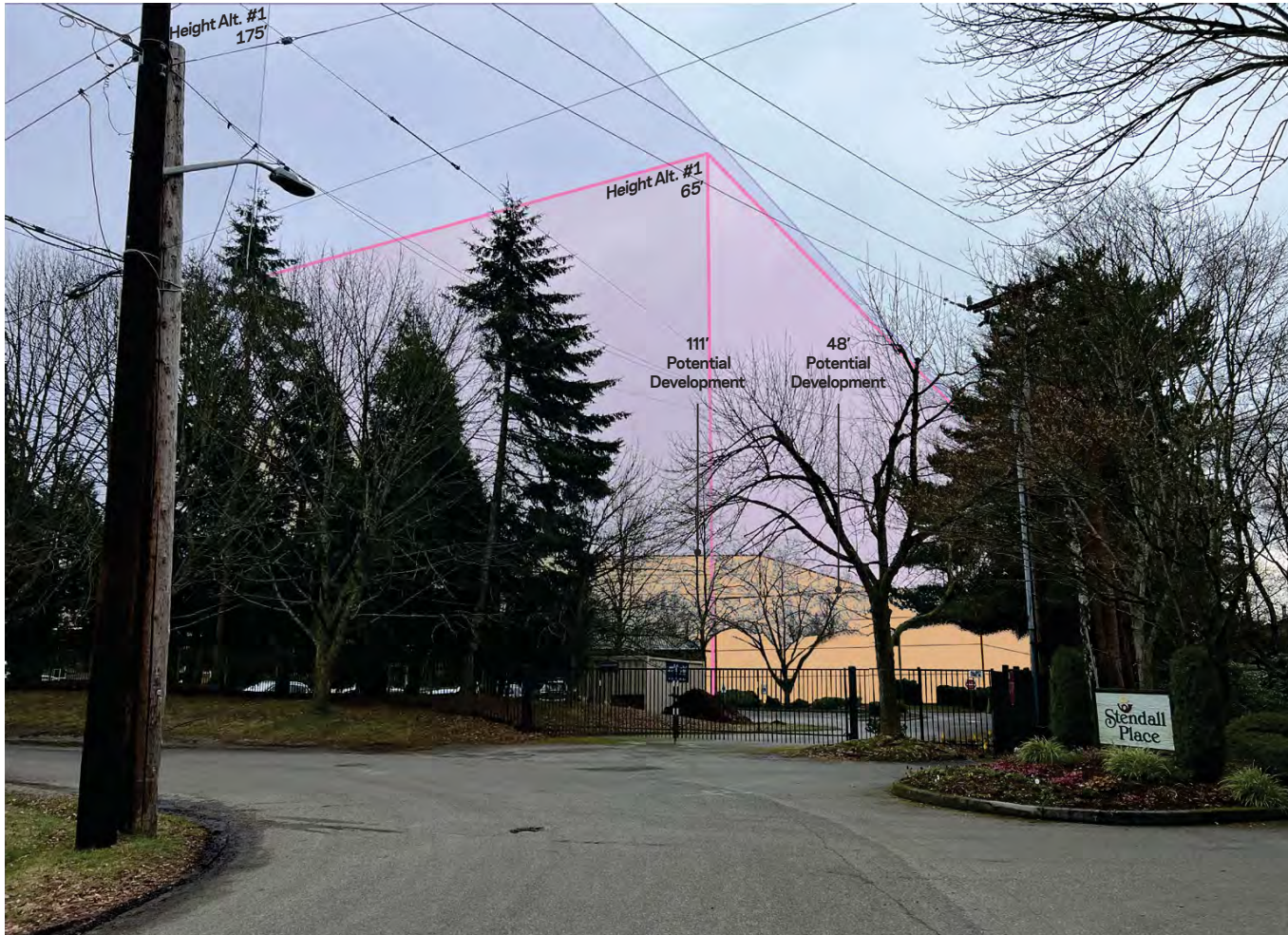
65' HEIGHT OVERLAY @ 30' SETBACK EAST FROM PROPERTY LINE; @40' EAST FROM CAMERA 175' HEIGHT OVERLAY @ 130' EAST FROM CAMERA (APPROX. 120' EAST FROM PROPERTY LINE) POTENTIAL DEVELOPMENT ALMOST 260' SOUTH FROM CAMERA
