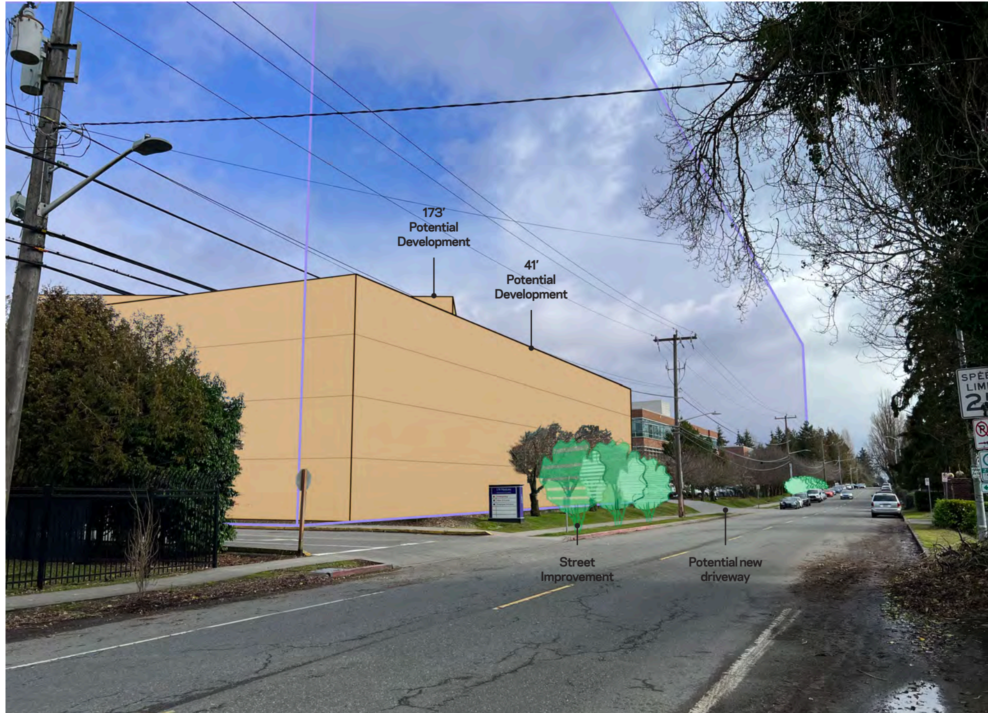
175' HEIGHT OVERLAY @100' EAST FROM CAMERA (APPROX. 40' EAST FROM PROPERTY LINE) POTENTIAL DEVELOPMENT ALMOST 110' EAST FROM CAMERA
