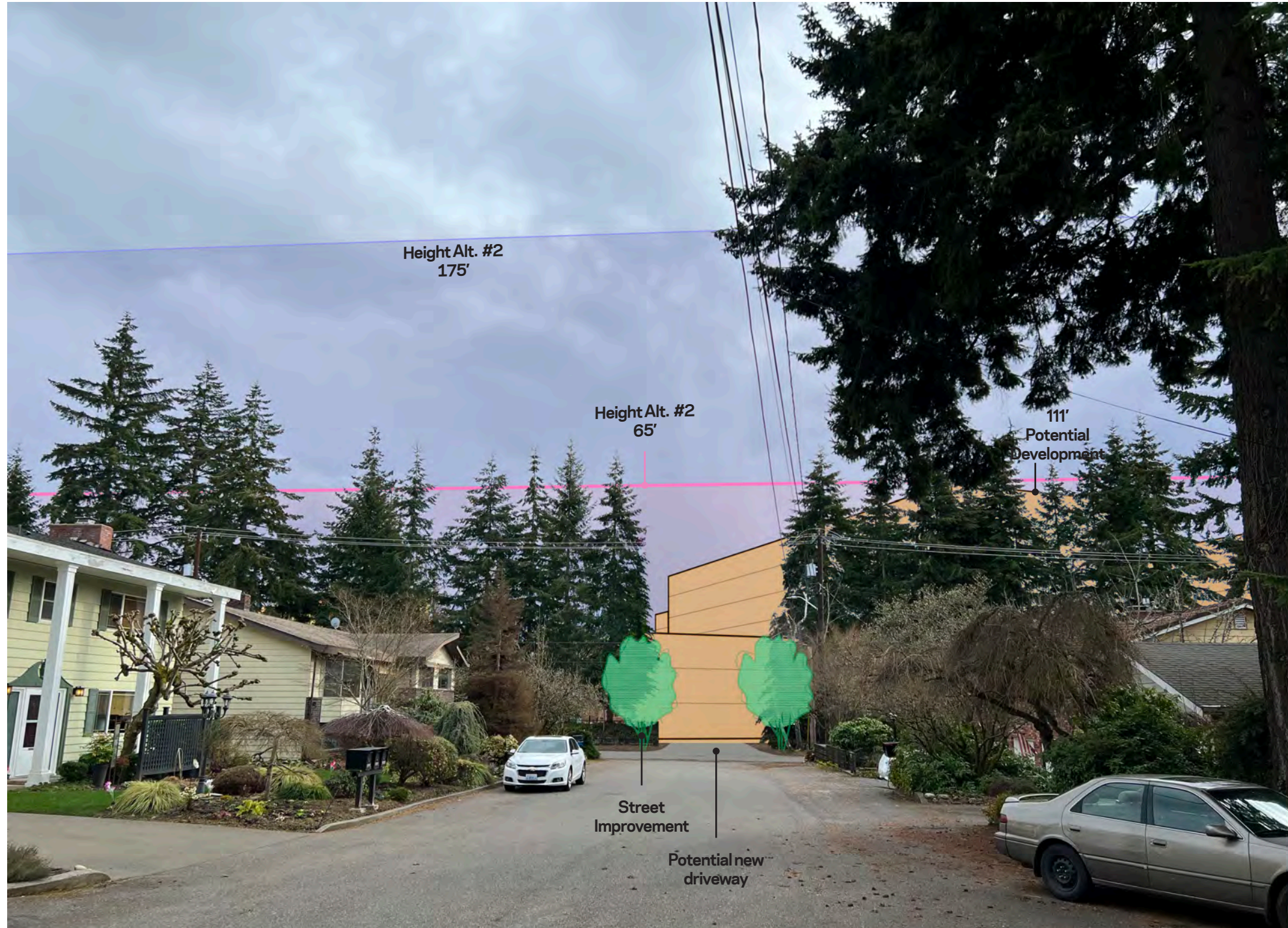
65' HEIGHT OVERLAY @ 20' SETBACK FROM PROPERTY LINE; @ 150' FROM CAMERA 175' HEIGHT OVERLAY @ 230' FROM CAMERA (APPROX. 100' FROM PROPERTY LINE) POTENTIAL DEVELOPMENT ALMOST 350' FROM CAMERA
