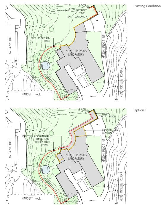
Option 1 – Security Fencing Near the Roof Edge
